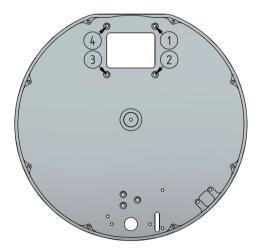
Attention – always use the screws supplied with the filter wheel. (M3×6 screw with countersink head). Longer screws may extend inside the camera head and may interfere with the camera shutter.
